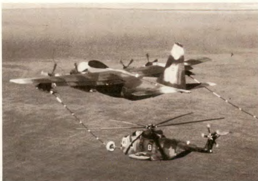
To complete its rescue mission safely, the HH-3 required air refueling by the HC-130 Hercules. First flown in 1964, the HC-130 Hercules is an extended-range, search and recovery version of the C-130 transport aircraft. Twenty HC-130s were modified with refueling drogue pods and associated plumbing for rescue missions. These aircraft are capable of refueling HH-3 and HH-53 helicopters in flight, thus greatly extending the helicopters' range.
