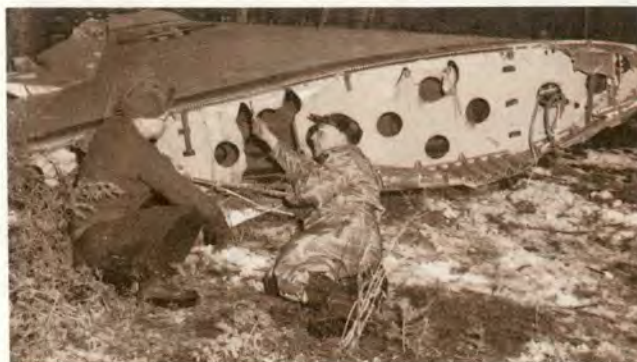
In the mid-1960's, the Air Force again advanced the scientific approach by using specialists during investigations. Here Sid Berman, renowned metallurgist, briefs Colonel G.A. Simeral, mishap board president, on damage to a C-47 wing torn off in 100 mph winds.
