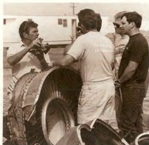
Safety officers and other potential aircraft mishap investigators receive hands-on training at the USAF Mishap Investigation Laboratory at Norton AFB, California. Better known as the Crash Lab, the facility not only has the complete remains of aircraft that have crashed, it also has individual pieces, such as wings or portions of engines, that are classic examples of different types of damage that lead investigators to discover the cause of mishaps. Here Professor Jack Hazlett leads student investigators through engine damage analysis.
